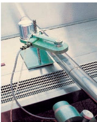
KI-discus containment test 1
