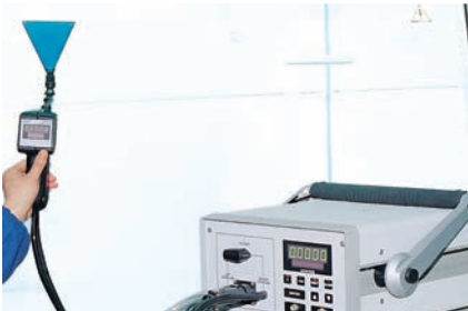
scan test for filters
